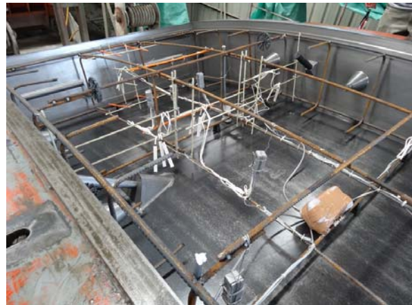
Figure 7. Instruments mounted in-situ
