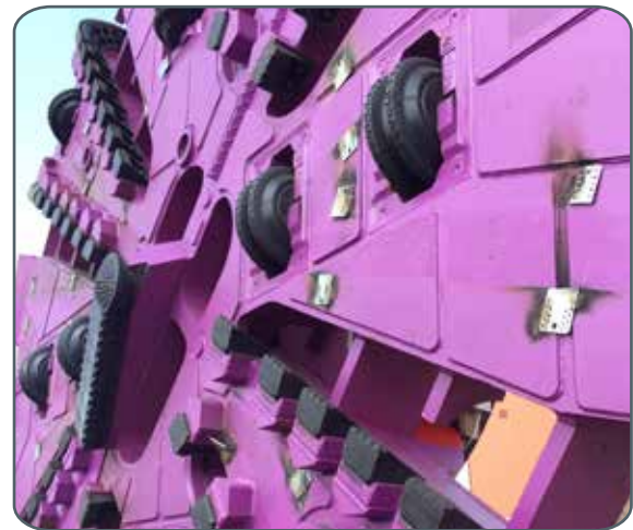
Image: Cutter head of one of Metro's Tunnel Boring Machines extending the Purple Line. Photo credit/courtesy of : Joe Linton/Streetsblog L.A.
